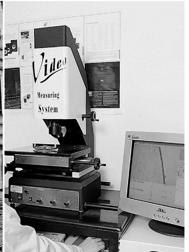
Precise Laser Video Measuring System 激光精密影像测试系统
