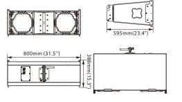
The medium to large sized weatherproof line array loudspeaker used in applications including sound reinforcement for Houses of Worship, Events, Stadiums, Theme Parks, Multifunctional Auditoriums, Schools, and Transit Terminals etc. Excellent for live, rental and portable outdoor sound reinforcement applications. The TLA Series line array loudspeaker delivers extraordinary performance where high speech intelligibility and natural sounding music is required at unmatched value.
