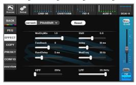
[ WetDryMix ]: Wet and dry mixing . 0: only input signal, 1: only tone effect signal .
