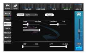
[ Delay ]: Delay, unit: ms. Input signal and feedback signal of delay.
