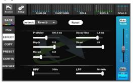
[ **PreDelay**]: The time interval between the front-reflection and the direct sound. The bigger the PreDelay, the bigger the space, on the contrary, shorter.
