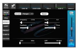
[ Frequency ]: Modulation frequency. Quick modulation frequency can cause one vibrato effect, but frequency shift will be caused if it is too fast.
