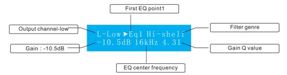
Press the channel choose key and choose the related channel need to be adjusted and press the Para key to choose the parameter which can be changed by the key of +/--.
