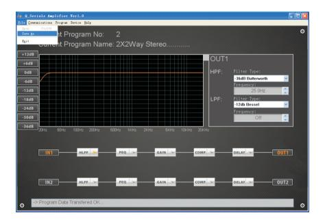
3.2>User also can save the adjusted parameters into the device directly Due storage space limit, total 50 programs can be saved through "Save as current program In Device" under "Program" menu. See below:
