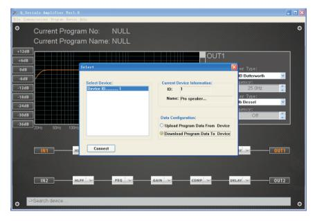
4.2> For the config files saved in the device, it can be recalled through "List Program & Recall" in "Program" menu, the software will read the data again and then update the display Automatically, see below:
