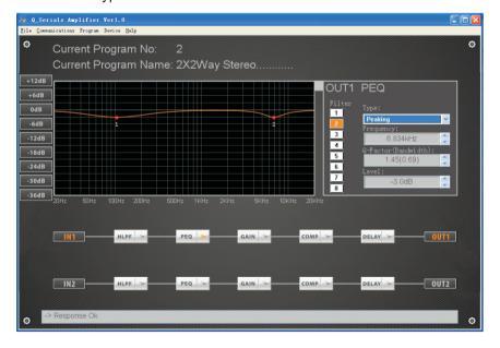
6.3>: The channel gain and volume adjustment, use mouse to click below "Gain" key, the right side of screen can select channel phase and adjust the volume output.
