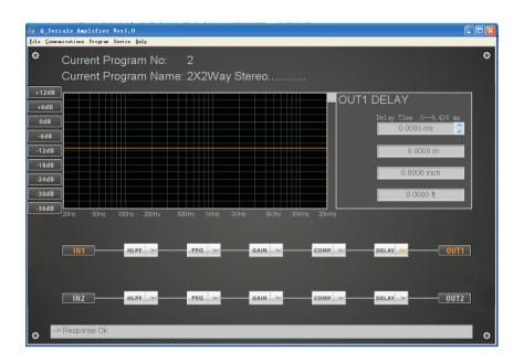
6.6> The data copy between channel 1 and channel 2, if channel 1 parameters are set up and channel 2 needs to same as channel 1, click "Copy all parameters from ch1 to ch2" under "Program" menu to realize.
