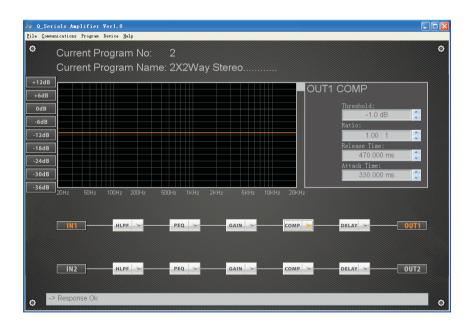
6.5> Channel delay time adjustment, use mouse to click below "DELAY" key, the right side of screen can adjust the delay time.
