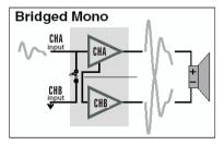
▲ Under the bridge mode, the output voltage is so high enough to make a electronic shock. Please power off the unit before operate it under bridge mode.
