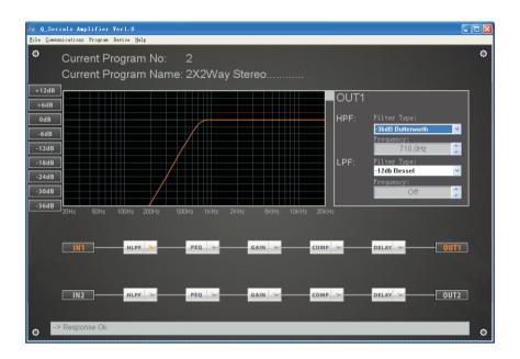
6.2> EQ filter adjustment: Choose below PEQ key, the right side of screen can select the type, frequency, Q value and level of filter. There are 8 EQ points for every channel, each EQ can set different filter type.
