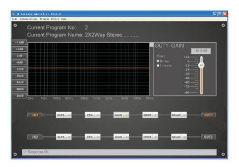
6.4> Channel power output compressor adjustment, use mouse to click below "COMP" key, the right side of screen can select compressor threshold, ratio, release time and attack time.
